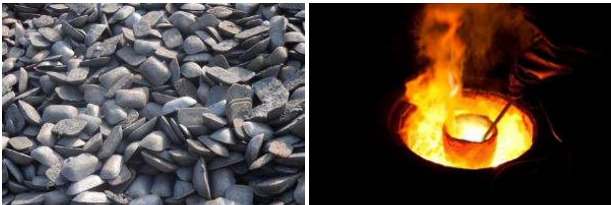
Figure 1.2-3.: Solid Pig Iron before being utilized in a foundry and liquid metal proceeding from pig iron melting
