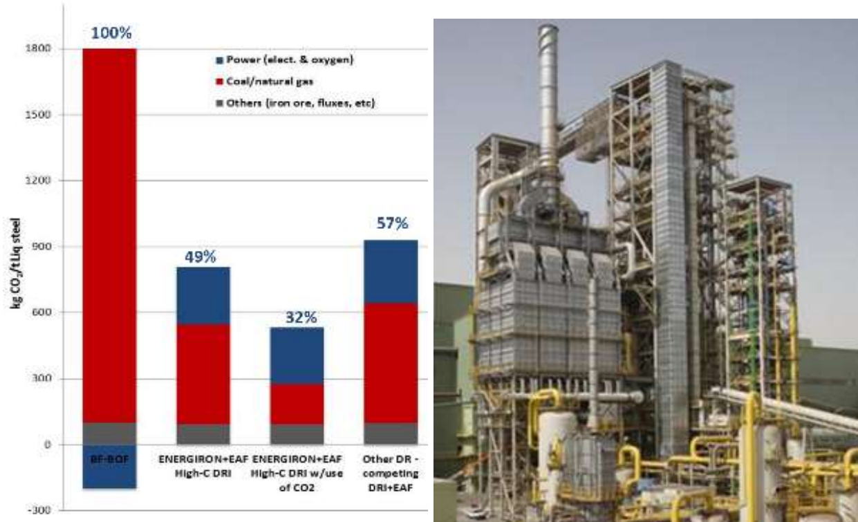
Figure 1.2-5: CO 2 emissions from different steelmaking routes showing that the process selected by PURE FONTE LTÉE has the lowest environmental footprint and photo of a CO 2 absorption plant
