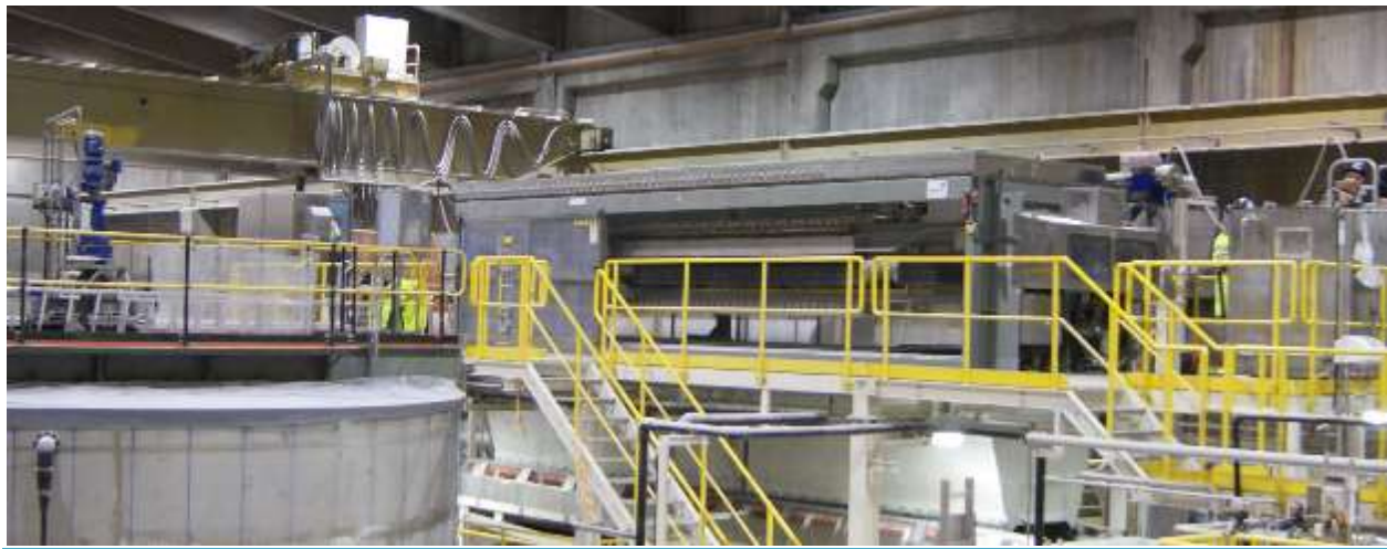
Figure 1.6-2.: photos of a FAST filter press by Tenova, used to remove dust from water [2]
