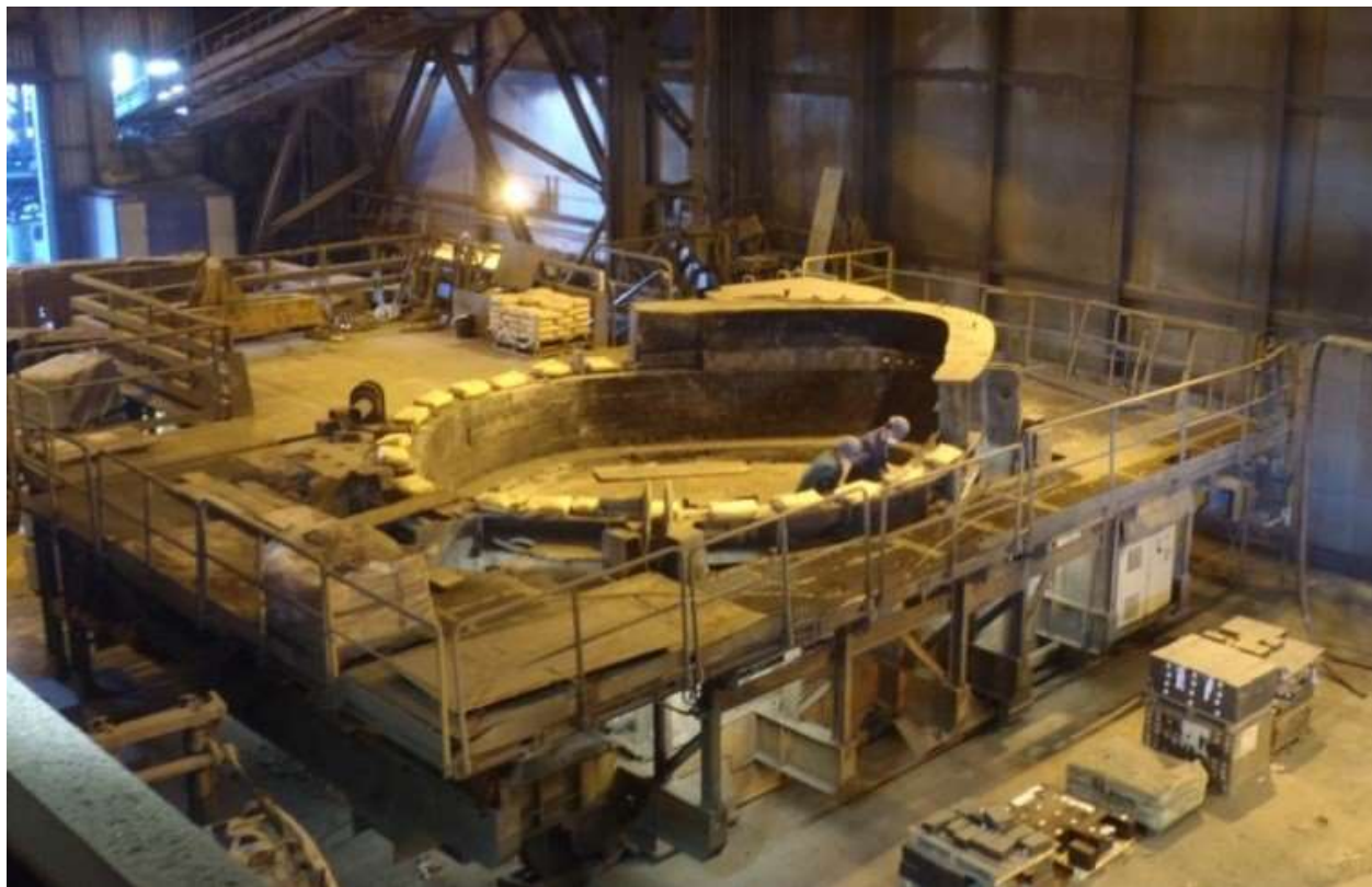
Figure 10.3-57.: Shell Maintenance Platform Area- For reference only
