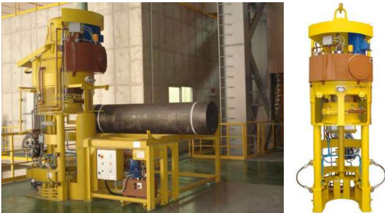
Figure 10.3-59.: photo of the electrode storage equipment and the electrode jointer machine
