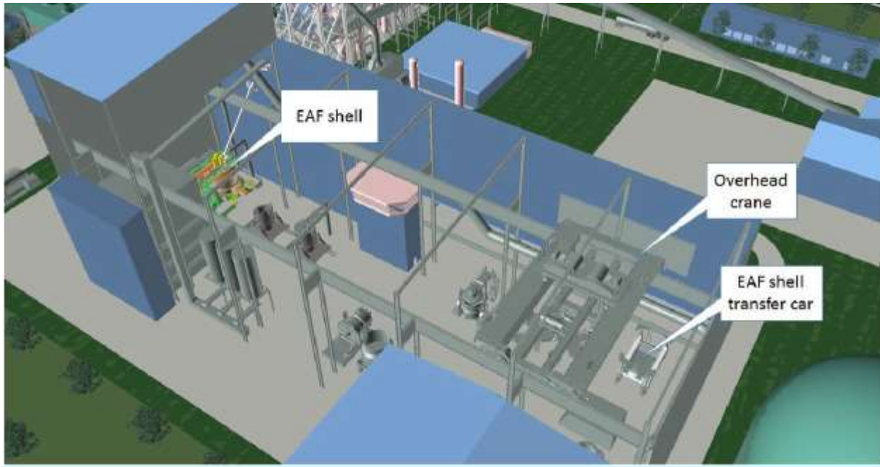
Figure 10.3-56.: position of the EAF shell transfer car at the north end of the main building
