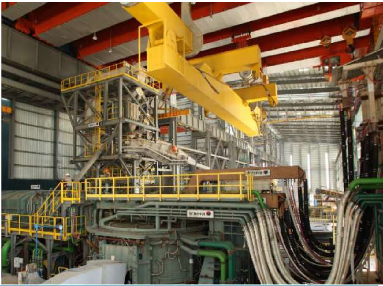
Figure 10.3-28.: a typical Tenova EAF
