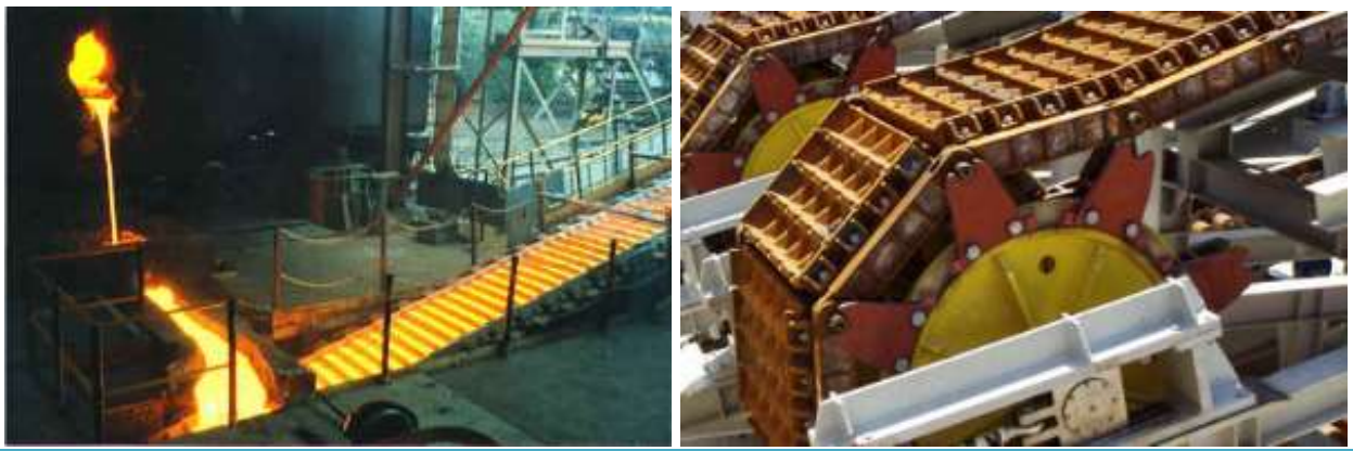
Figure 1.5-15.: Pouring iron at ISCOR in Pretoria [12] and photos of Paul Wurth pig casting machines [13]
