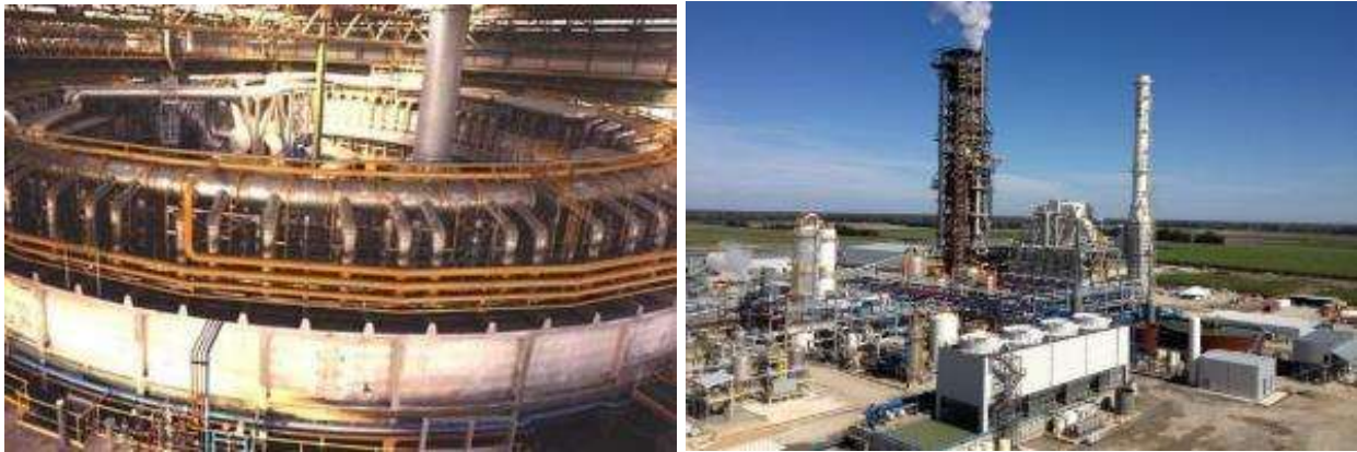
Figure 1.5-1: photos of a Rotary Hearth Furnace (RHF) made by Tenova Core Inc. [1] and the Energiron ® plant of Nucor Louisiana by Tenova HYL [2]
