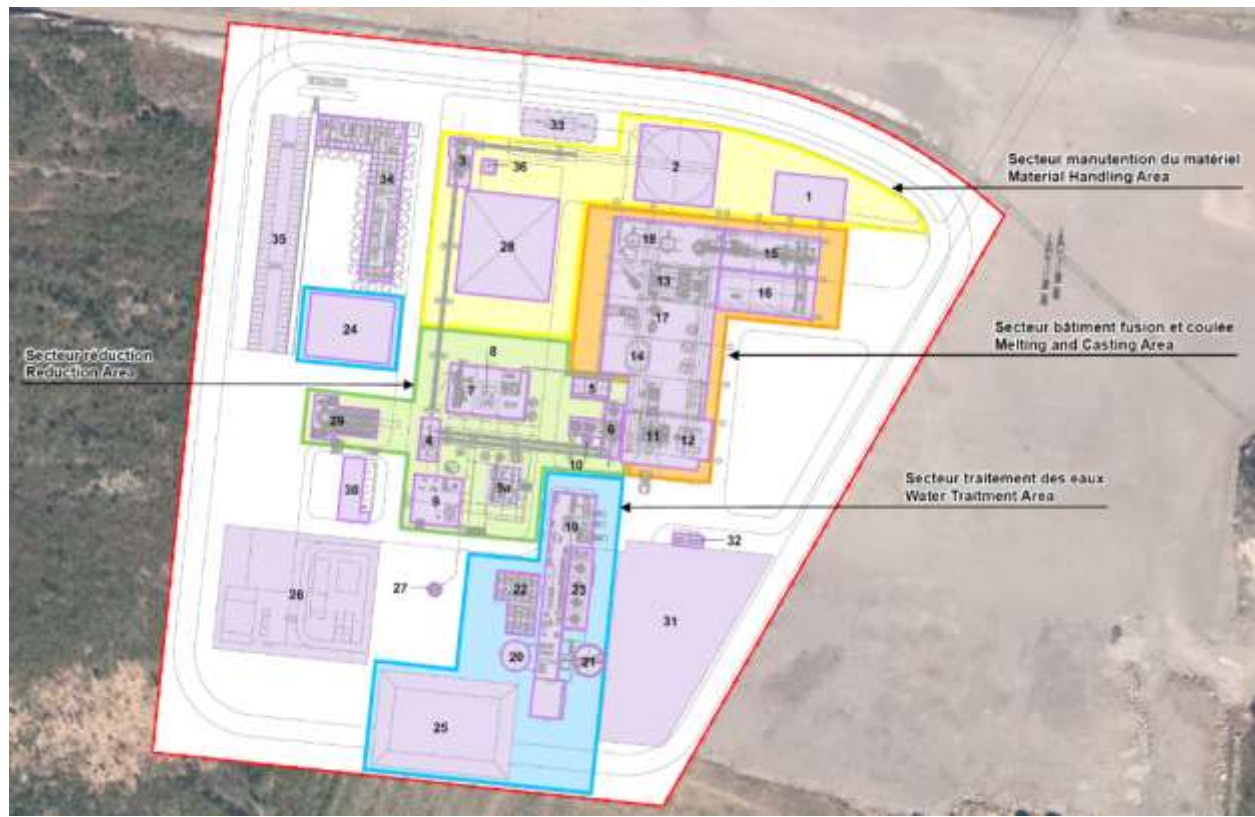
Figure 1.4-5.: Identification of buildings and other plant elements [2]
